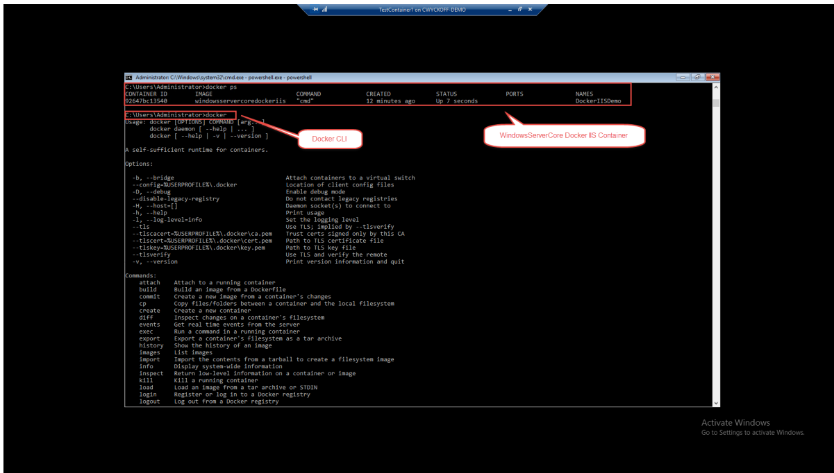
Figure 13: Docker Container and Docker CLI
